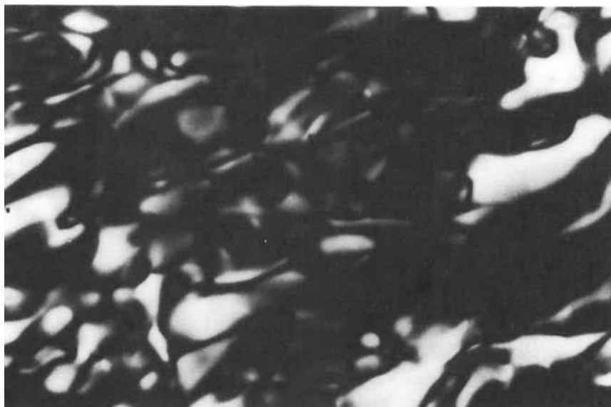
Fig.2. A nematic lyotropic mesophase formed by SDDS/PDE/H 2 O, composed of 20.02% SDDS, 12.02% PDE and 67.96 % H 2 O (sample A1).
